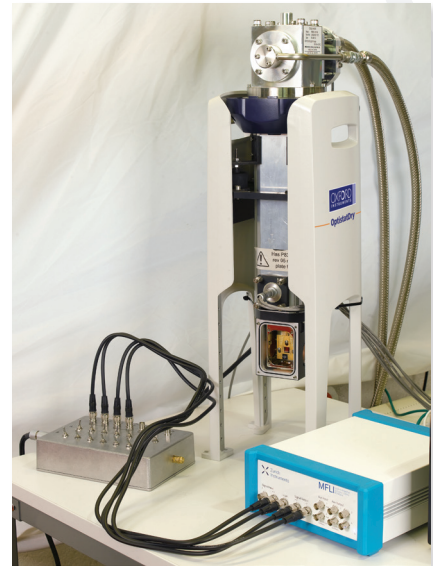
Figure 1. Set-up of MFLI lock-in amplifier and Optistat ™Dry Cryofree® cryostat
